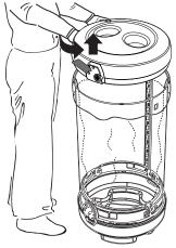
1.3 With the key still in position, turn hood counter-clockwise, then lift hood off. Remove the key.
