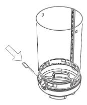
2.1 Remove hood as (1) above, remove sack if present. Insert the plastic key into the lock.
