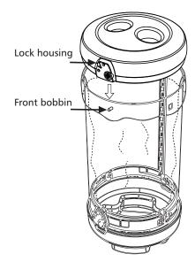
**1.5** Place the hood onto the body and align the lock housing with the front bobbin by turning the hood. Push the hood firmly downward to automatically lock the unit.
