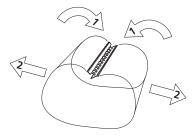
2.3 To disassemble the body place on a well-protected and soft surface, joint uppermost. Push down either side of the interlock to disconnect the tabs, and allow the sheet to spring flat.
